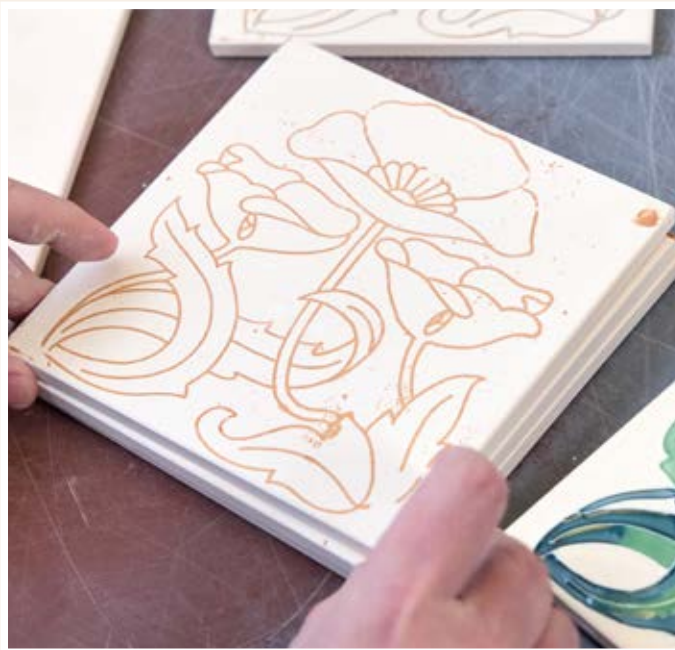
▲ The pattern is stencilled onto the blank tile biscuit.
