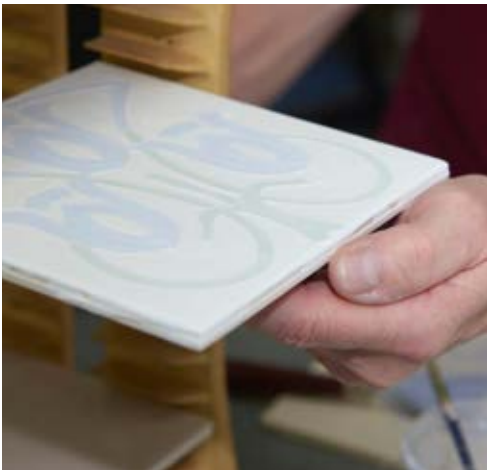
▲ When all the colours have been applied, the tile is inspected, loaded into a crank and then left to dry, ready for firing
