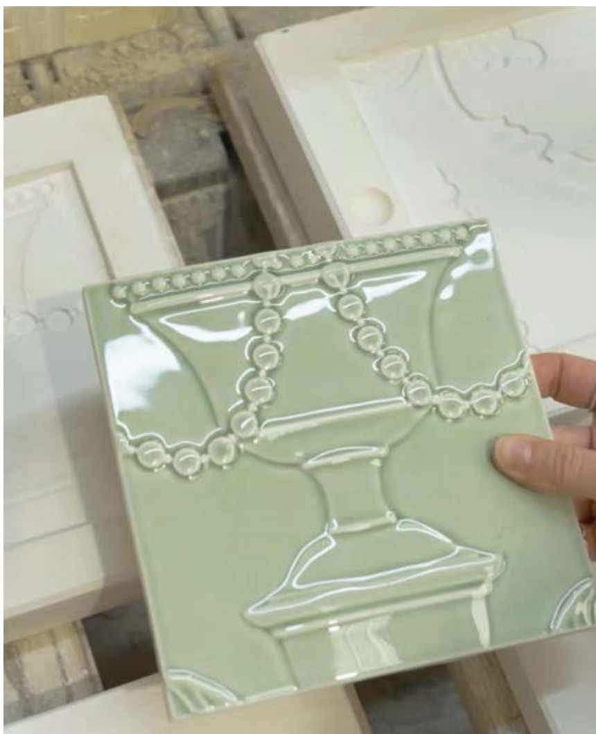
▲ Bespoke glazed moulding with plaster moulds
